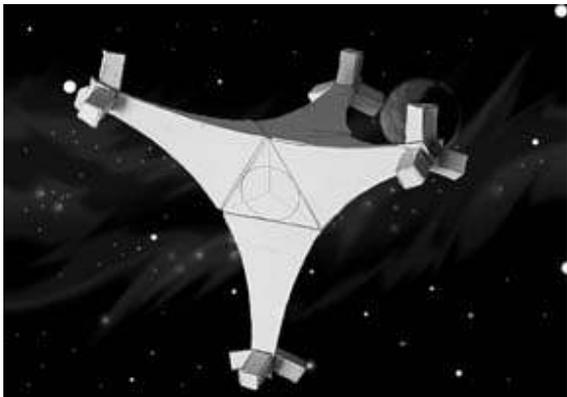
Robot for zero-gravity operations. They are tetrahedral, able to send bursts of gas from their corners to move and orient themselves.
