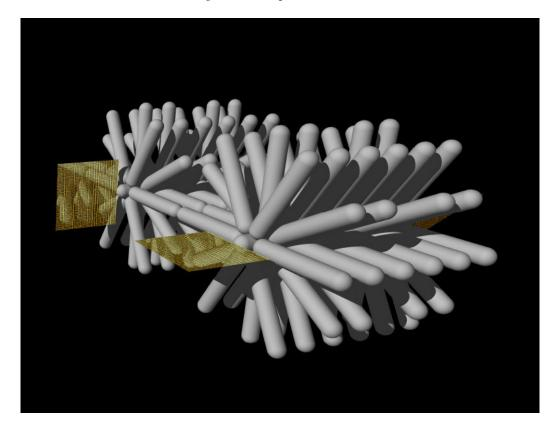
In the above example, the barge Navas del Pinar consists of 124 tanks arranged in bundles around central tanks and connected through endcaps. Radiators are placed at the sides, providing cooling for the system. Fullerene cables connect the tanks and hold them in place; the whole barge can be towed at 0.03 G without risk. Total width 110 meters (plus 120 meters of radiators), length 240 meters. There is space for 5,000 inhabitants, divided into a number of barrios separated by pressure doors.
