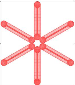
The spherical endcaps can be equipped with openings allowing more tanks to be connected. A common design is "stars", where six tanks are placed as a star. This structure can be
